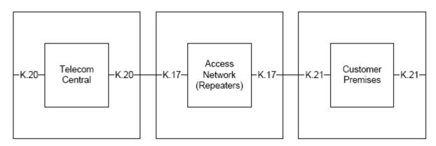
Each recommendation has a list of test schemas, time of emission, voltage and current limits. These tests allow a simulation of events that could happen on a real network. Recommendations only define borders, but they could be too low for real life. That's why good xDSL equipment must have better protection then defined in the ITU standard.
