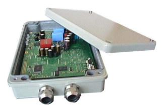
For harsh environments and outdoor use FlexDSL Orion 2 Repeaters are also available in cost effective and high profile aluminum enclosures, extending single or dual pair SHDSL (TC-PAM16/32). It offers Ethernet add/drop functionality (10/100BT, Bridge) and is protected by an IP-67 aluminum housing. The repeater can be powered locally or remotely over the DSL line. Therefore, it is configurable as power "end-point" or "pass-through".
