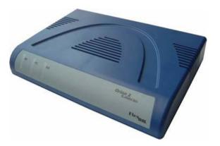
The most common FlexDSL Orion 2 Repeater extends single pair SHDSL (TC-PAM16/32) up to 5.7Mbps. It offers Ethernet add/drop functionality (10/100BT, Bridge) and comes in a plastic desktop housing. The repeater can be powered locally or remotely over the DSL line. Therefore it is configurable as power "end-point" terminating power transmitted over the DSL line, or power "pass-through", passing power on to another repeater or CPE device on the DSL line.
