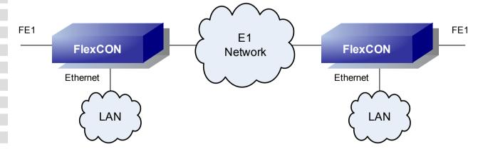
FlexCON also could be used for Ethernet + Fractional E1 (FE1) transmission over E1 network. This application is important when Carrier has limited E1 channels in core network but customers want Ethernet data transmission as well. FlexCON allows flexible bandwidth selection with 64 kbit/s step
