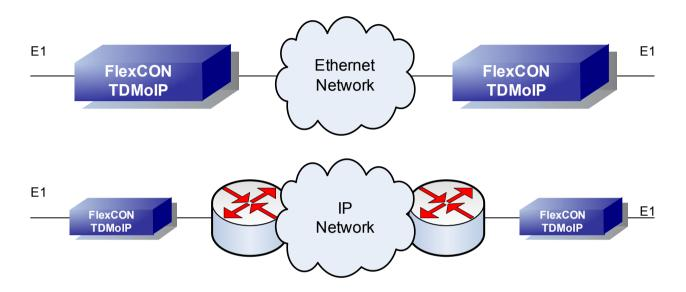
FlexCON TDMoIP units were designet for single E1 channel transmission over packet network. They support all important technology like VLAN and ToS. FlexCON could send TDM data in UDP or RAW formats. If Packet network has one or more routers, UDP protocol must be selected. FlexCON modules have internal G.703 clock generation and recovery features as well as jitter suppression methods.
