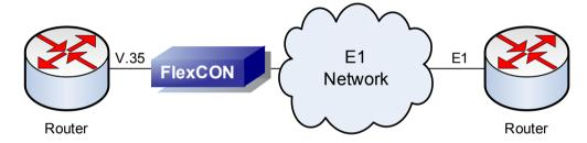
Several ISPs routers have E1 data interface with framed structure while old V.35 interface still popular for SOHO routers. FlexCON could be used for such interconnection.
