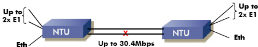
Point-to-Point Bonding Application with Failure Protection
