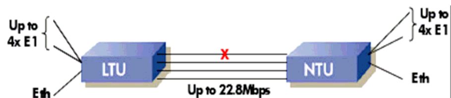
Point-to-Point Bonding Application with Failure Protection
